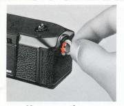
1. Unscrew the battery chamber locking screw 2.
