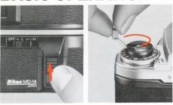
**13.** Rewind the film. Push the rewind slide ① up and then rewind the film manually by turning the camera's rewind crank.
