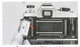
**14.** Remove the film cartridge. Unload the film in the normal manner, avoiding direct sunlight.
